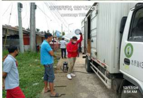
The Opacimeter setup process, including the start-up, insertion of the probe, reading emission levels through controlled pedaling, and printing out the test results.
